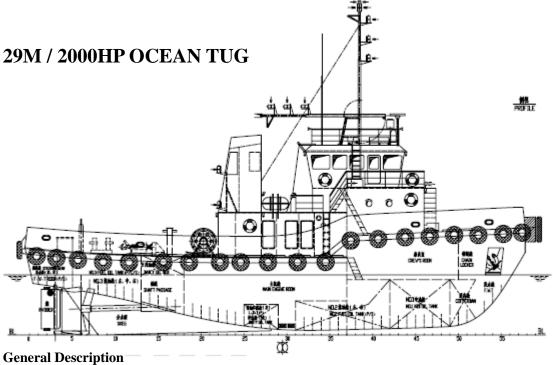
The vessel is to be all welded steel construction with twin diesel engines, twin fixed pitch propellers for towing, pushing offshore supply and other related duties. It will be classed to ABS for towing services of unrestricted navigation.
